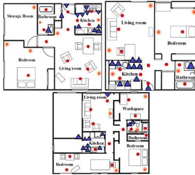
Figure 47: Three smart home testbeds - floorplan. Red circles and blue triangles represent PIRs and magnetic door sensors respectively [Nazerfard and Cook, 2015].
