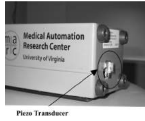
Figure 26: Floor-vibration sensor for fall detection [Alwan et al., 2006].
